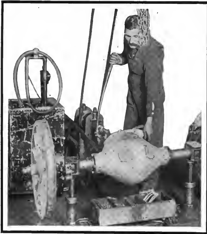
After brakes and wheels have been attached, the completed bridge assembly is filled with oil and tested under belt
